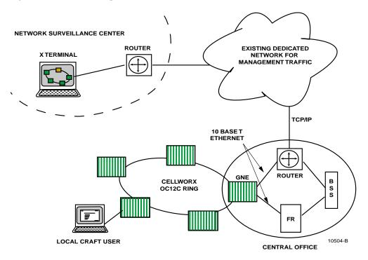
Figure 1-14. Remote X-Terminal Operations
